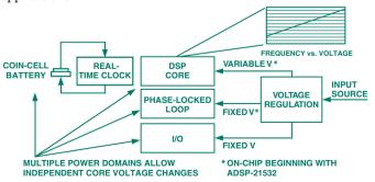
Figure 5. Illustration of multiple power domains within the Blackfin DSP.
