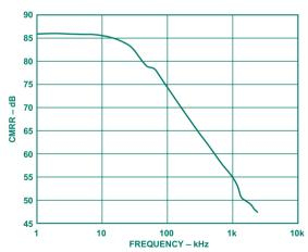
Figure 6. Typical CMR vs. frequency—AD7677/AD8021 combination.
