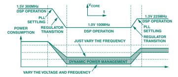
Figure 1. Effects of V and F changes on power consumption.
