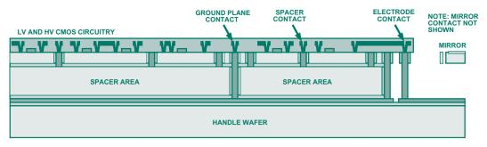
Figure 3. Analog Devices optical iMEMS process—optical mirror fabrication with integrated circuitry.
