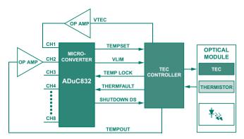
Figure 3. The MicroConverter sets the TEC target temperature and monitors its performance.
