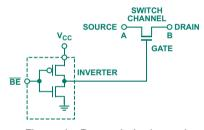
Figure 1. Bus switch channel.
