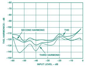
Figure 1. THD, second and third harmonics vs. input level for AD7671/AD8021 ADC/driver combination.
