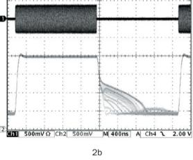
Figure 2. Tails at the output of a log amp in response to RF bursts.
