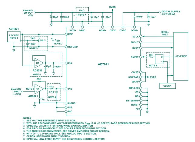
Figure 2. A single-ended-input 16-bit data acquisition system. References in Notes are to sections of the AD7671 data sheet.
