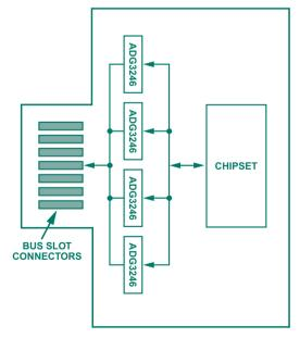
Figure 10. Hot swapping with the ADG3246 bus switch.
