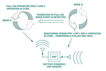
Figure 4. Sample DSP application with different operating modes.
