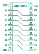
Figure 12. Flow-through pin arrangement.
