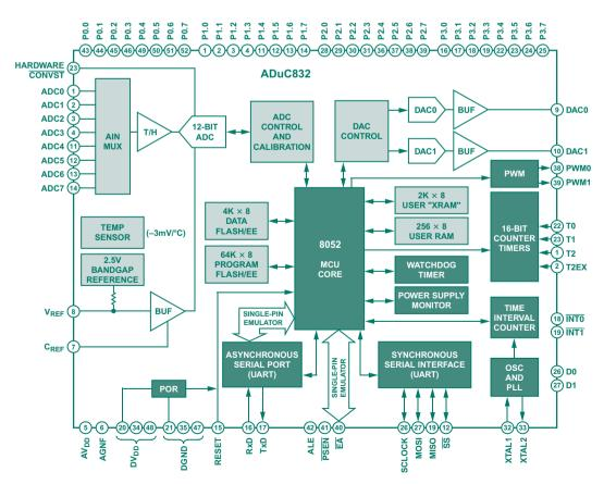
Figure 2. MicroConverter block diagram.
