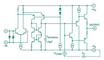
Figure 7. AD8021 simplified schematic.
