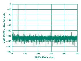
Figure 3. FFT plot of AD7671/AD8021 combination.
