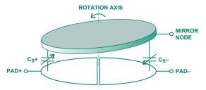
Figure 1. Capacitive bridge established by mirror structure.
